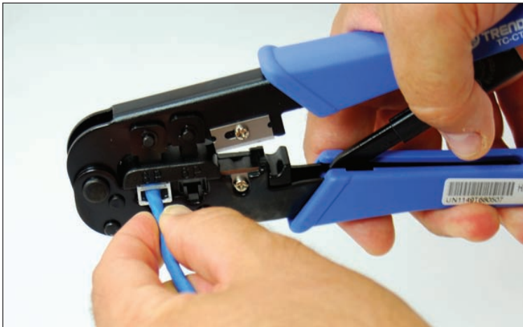
Figure 8-47 Use the crimper to crimp the connector to the cable
